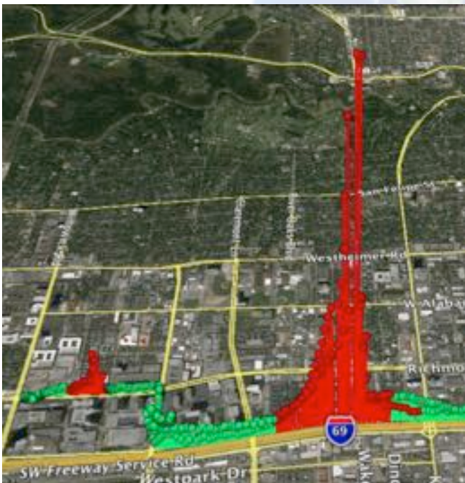
Red indicates highly correlated ethane to methane concentrations in the Houston area on two different passes through the same region at highway speeds, identifying a persistent natural gas leak.
