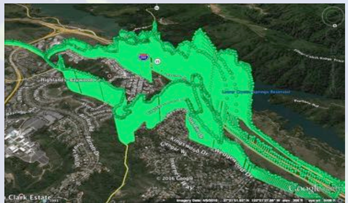
Green indicates the spatial mapping of a significant methane-only plume on repeated passes over several hours, in this case from a nearby landfill, unambiguously ruling out natural gas as the source.
