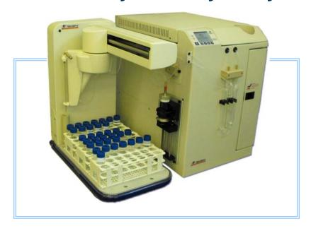
Tekran Instrument Corporation introduces the new *Tekran 2700 Methyl Mercury Auto-Analysis System*. The 2700 has been designed to give analytical laboratories and researches an alternative to the time consuming and complex manual method (*EPA 1630*). The *Tekran 2700* accomplishes this in a fully integrated, self contained compact unit (*MDL=0.002 ng/L*), operated via state of the art software.
